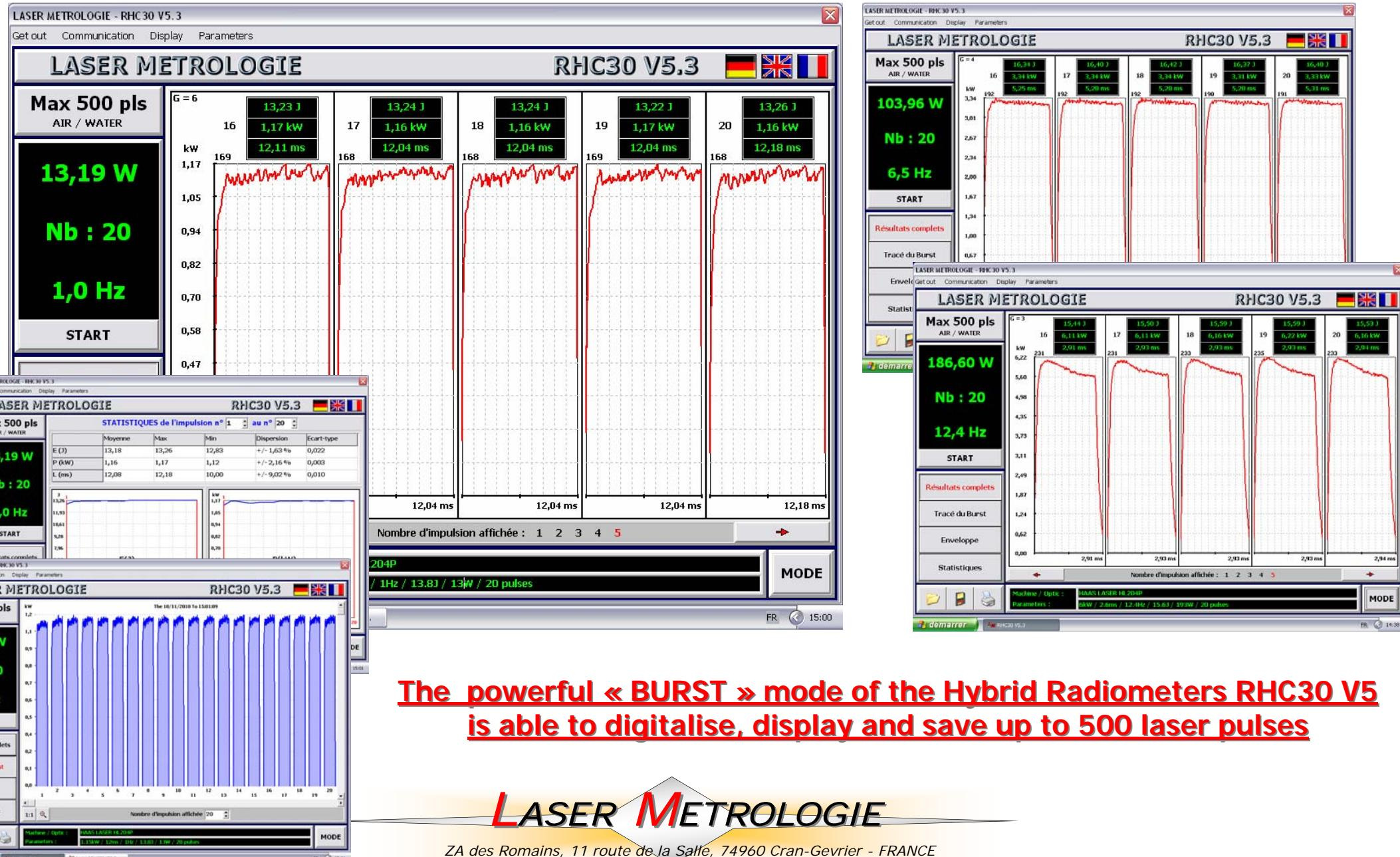
The powerful « BURST » mode of the Hybrid Radiometers RHC30 V5 is able to digitalise, display and save up to 500 laser pulses
